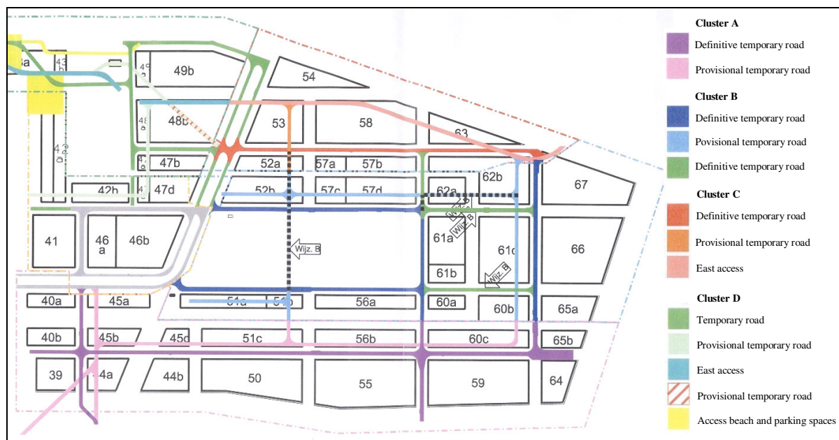
Figure 9: phasing temporary roads on IJburg East (Ingenieursbureau Amsterdam April 2005)
