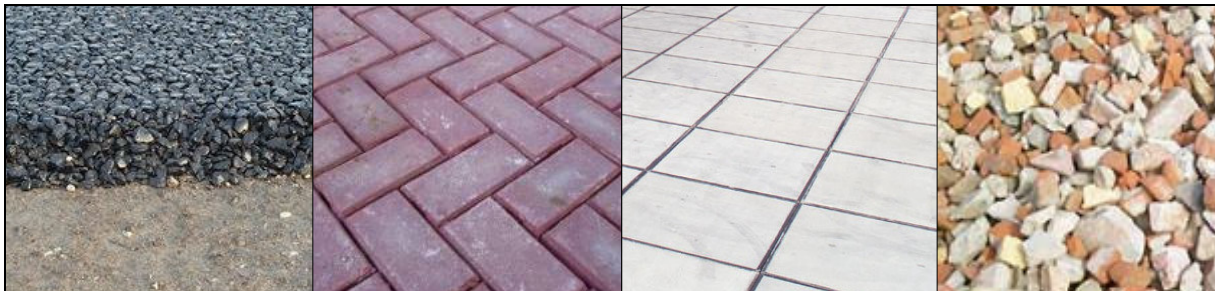
Figure 53: asphalt, small elements, prefabricated concrete plates and unpaved road.
